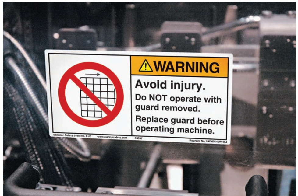
Figure 1: “Do Not Operate with Guards Removed/Gears Beneath” safety symbol (at left) and a best practice safety label designed to warn against operating machinery without the proper guard in place (at right). (Label design ©Clarion Safety Systems.)
