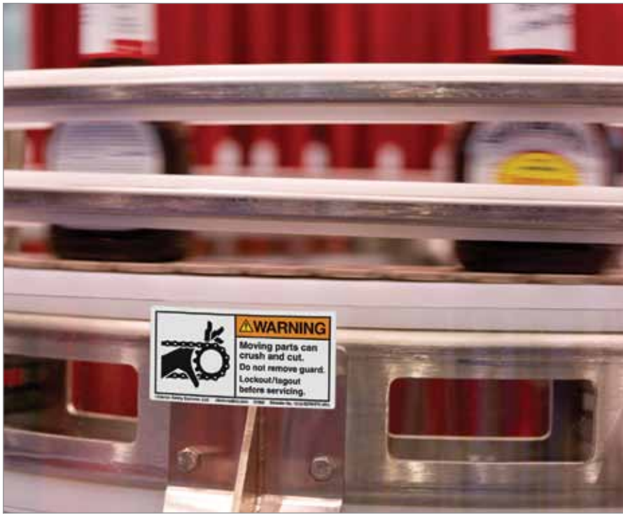
Correct: A safety label placed at the point of possible interaction with a mechanical hazard.
