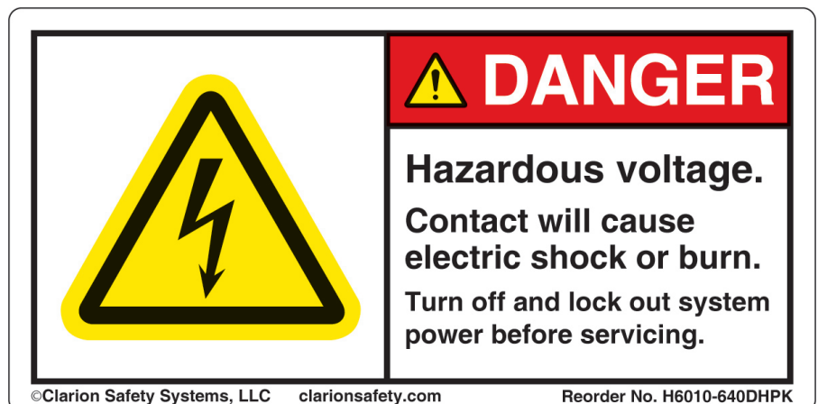
Figure 1: Example of an ANSI 2011 Z535.4 electrical hazard product safety label. (Design ©2014 Clarion Safety Systems. All rights reserved.)
