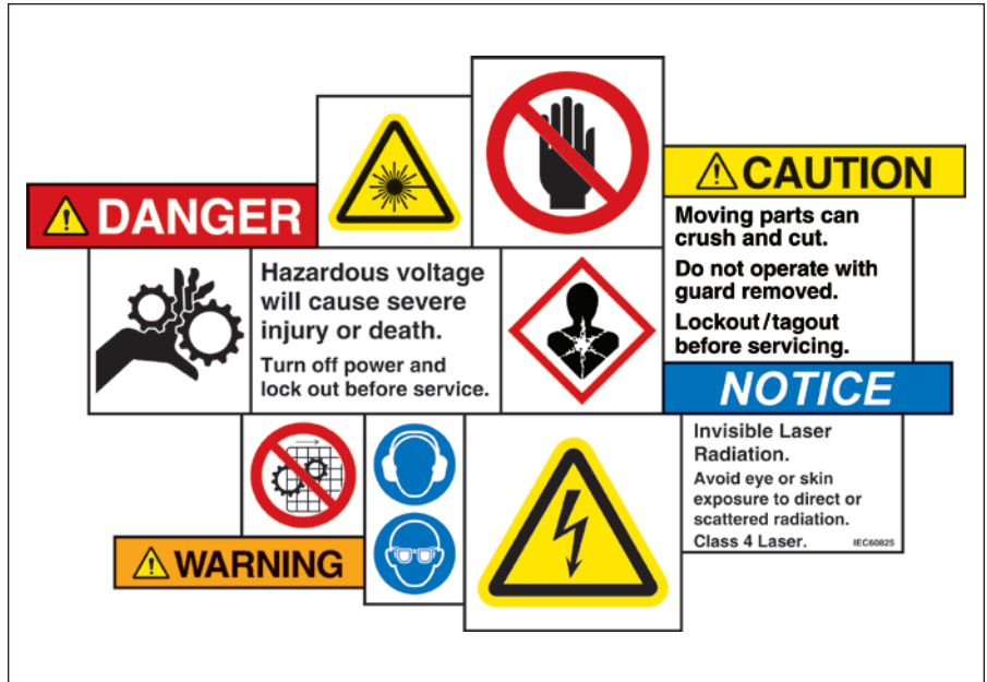
Figure 2: A compilation of all the different elements (from signal words to text messages to symbols) that must be considered, and brought together cohesively, when designing effective product safety labels.
